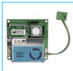
Air Quality Sensor (Co2/Humidity/VOC)
